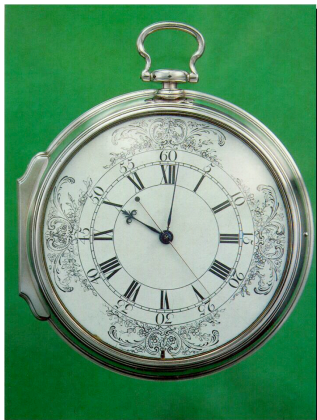
Figure 2. Harrison’s 1759 watch ‘H4’ for navigation at sea
